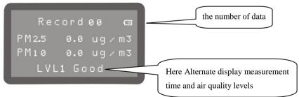
In Record Mode, if you want to check the data record of timing measurement, please press UP/ DOWN button to find the one which you want.
