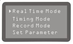
Press "UP" Key or "DOWN" Key to select "Real Time Mode" or "Timing Mode" or "Record Mode" or "Set Parameter" and Press "ENTER" Key to enter the corresponding mode.
